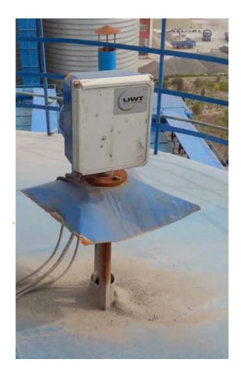
UWT measuring technology will always provide a professional solution in terms of precision and process reliability to support a cement production facility. In order to optimise the precise weighing and dosing of varying materials, it is vital that the measuring devices offer adjustable sensitivity. As a result, UWT sensors easily detect DK values from 1.5 or bulk density below 5 g/L (0.3 lb/ft<sup>3</sup>)
